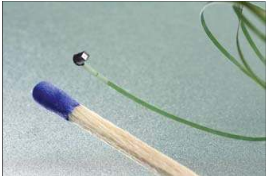
The NanEye family of image sensors is suitable for integration into endoscopy and surgical robot applications.
